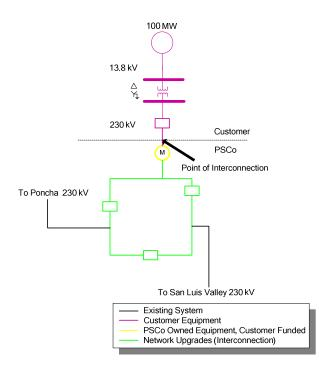
Figure 1a. Preliminary One-Line of the Proposed 100 MW Generating Facility
